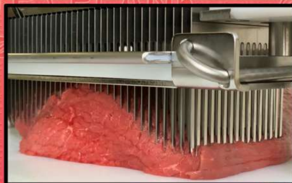
Penetration of the blades into the meat
